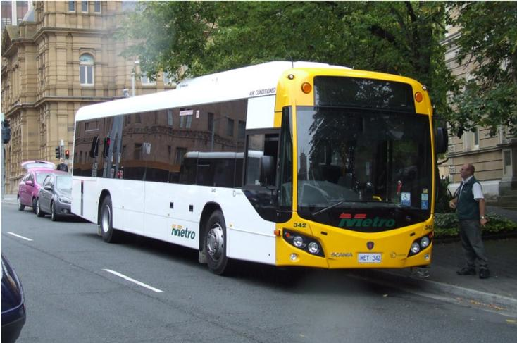
*CENTRE: BUS 342 is one of the latest batch of buses for Metro, Hobart being a 2014 Customs CB80 bodied Scania K280UB. (Bruce Tilley)*
